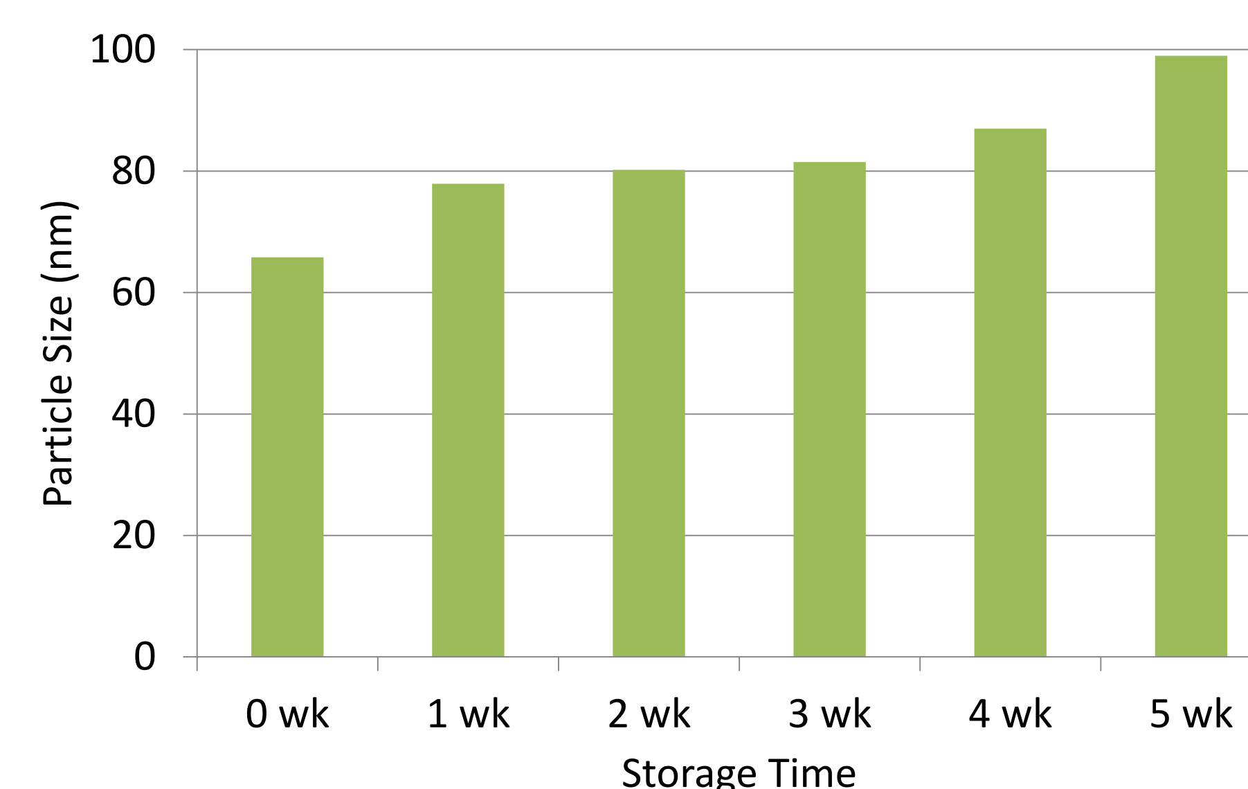
Figure 2. Particle size distribution of nano-emulsion prepared with 95%-pure lutein during storage
