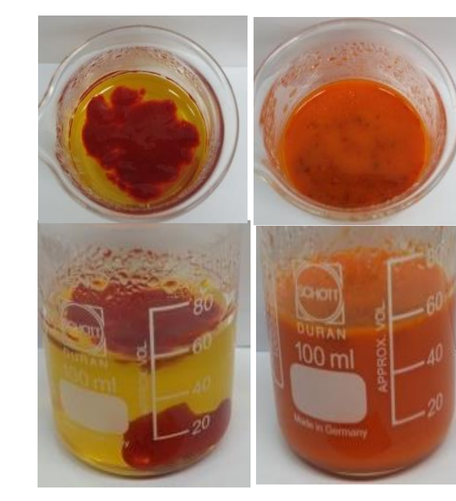
Figure 5. Pre-mixture of lutein (20% purity) with PG (left) and lutein:MCT (right) (1:1 w/w)
